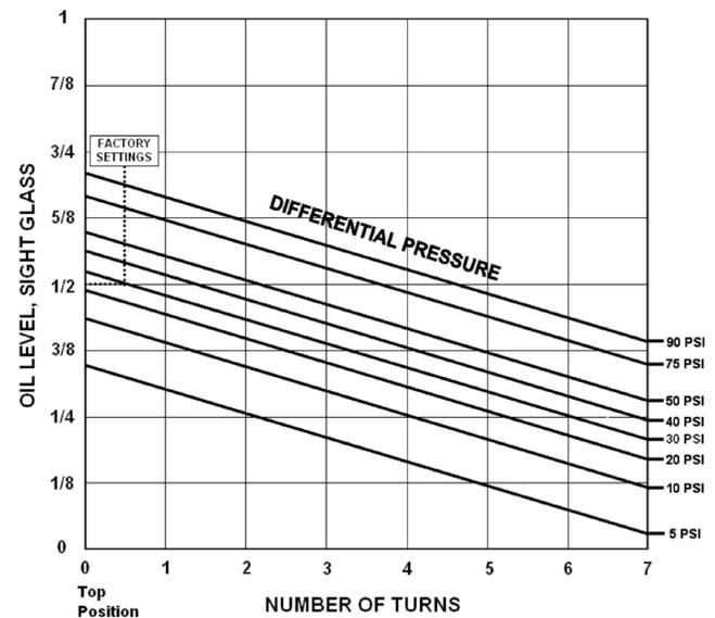
Note: Data obtained using POE lubricant at 86°F with a 1 inch diameter sight glass.
